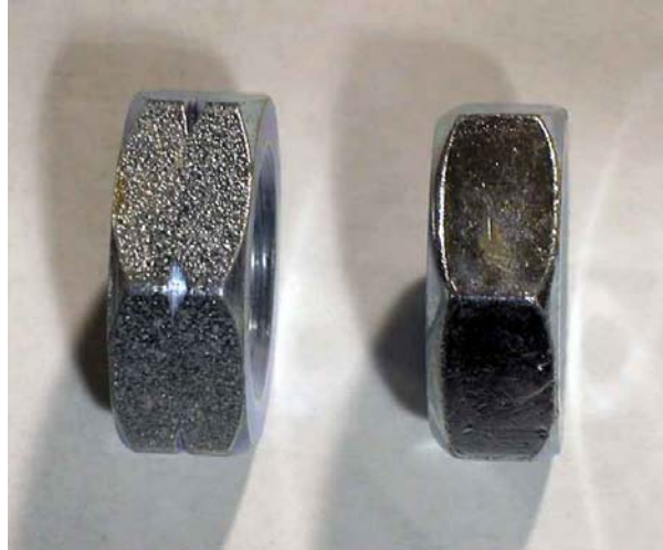
Jam Nuts, not marking on left hand thread jam nuts
