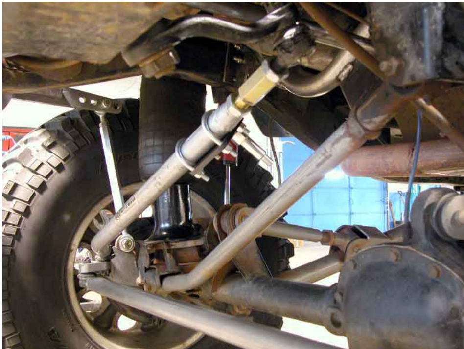
Steering Stabilizer Bracket installed
