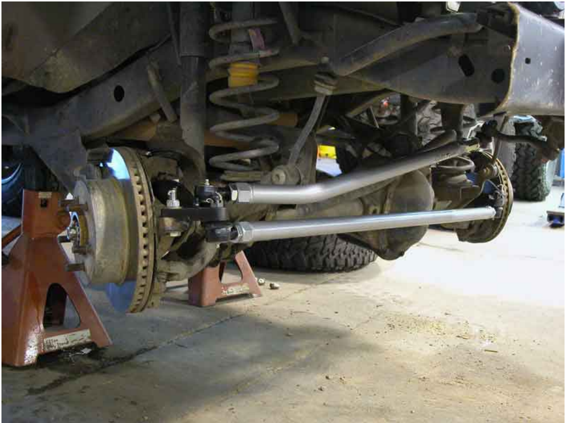
Finished assembly, note the position of the draglink.
