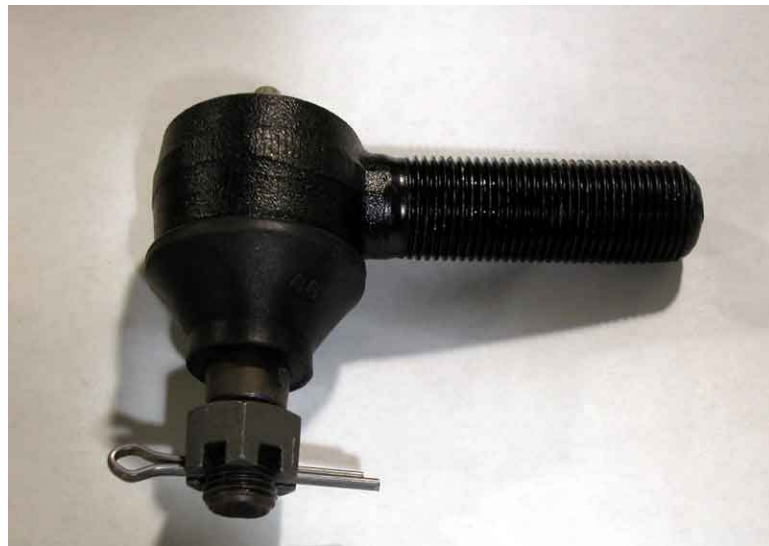
Tie Rod shown assembled. Note position of cotter pin.
