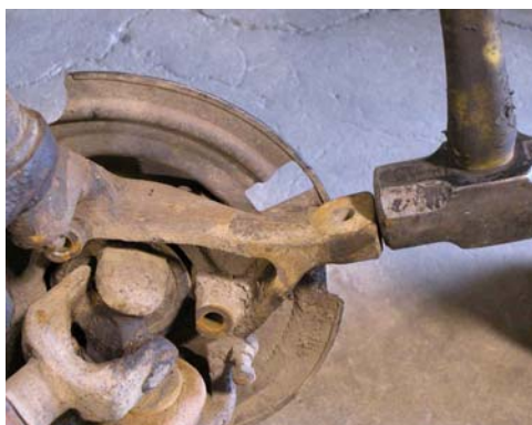
Hammer showing the proper position to break the taper free.
