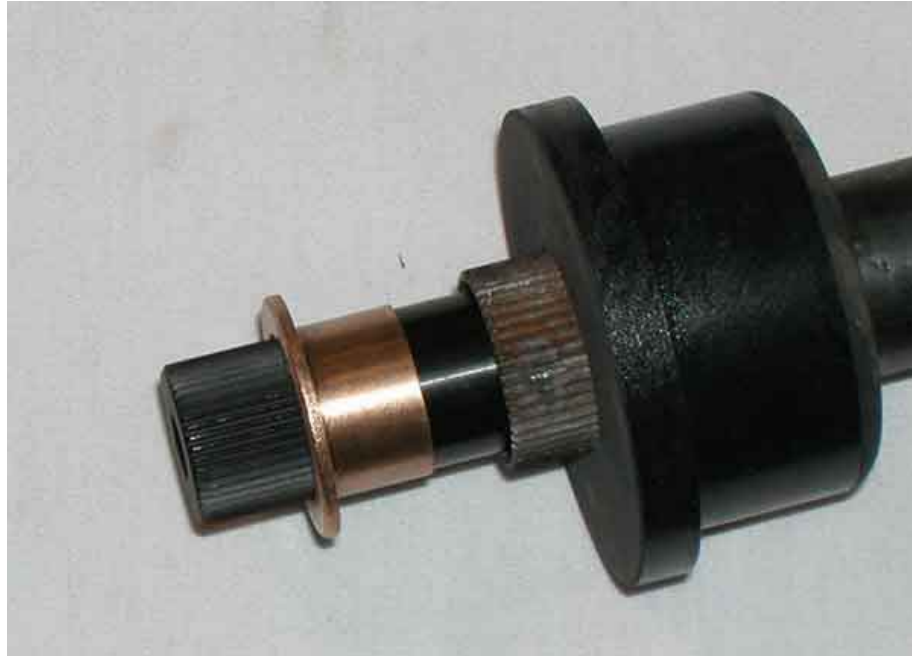
Figure 5 Brass Bushing Install Direction
