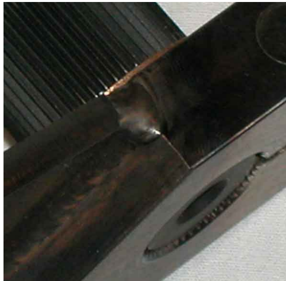
Figure 7 Proper Shaft Engagement
