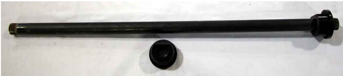
Figure 3 Torsion tube and bushings
