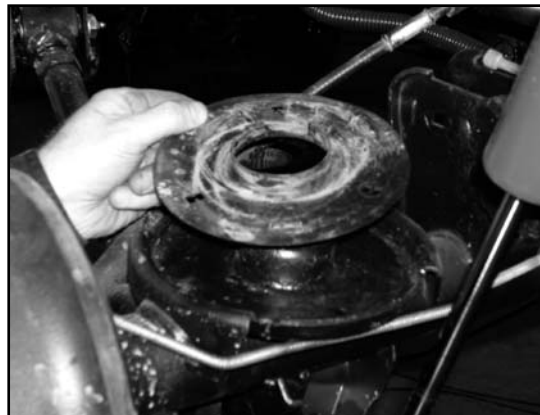
Figure 13.3: Removal of Lower Mount Insert
