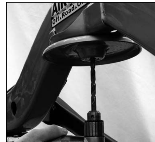
Figure 13.4 Drill upper bumpstop mount threads to 3/8"
