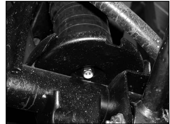
Figure 14.4 Install nut on lower stud
