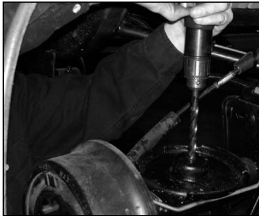
Figure 14.2 Drilling 1/2” Hole in Center of Spring Pad
