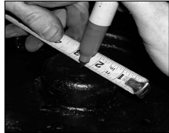
Figure 14.1 Marking Center of Lower Pad, need not be perfect, just as close to center as possible
