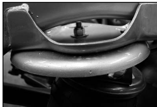
Figure 14.3 Install washer and nut on top mount
