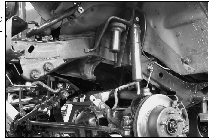
FIGURE 10.1 FRONT LEFT SUSPENSION WITH TRACKBAR AND COIL SPRING REMOVED, SWAYBAR DISCONNECTED
