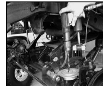
FIGURE 10.3 PLACE AiROCK LOWER FRONT MOUNT OVER SPRING PAD AND MARK FOR DRILLING 1/2" HOLE
