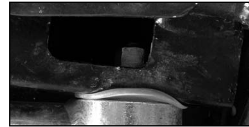
FIGURE 12.1 TRACK BAR BRACKET BOTTOM VIEW, NUT MUST BE INSERTED THRU THE SLOT
