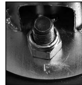
FIGURE 11.5 FRONT UPPER MOUNT MARKED WITH “F” POSITION THIS TOWARDS THE FRONT OF VEHICLE
