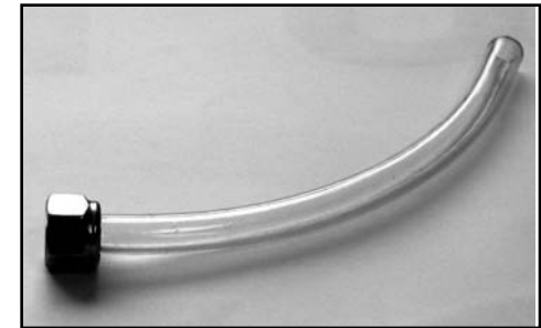
FIGURE 12.2 PLACE HOSE INTO NON-NYLOCK END OF NUT, PUSH THRU UNTILL ENOUGH THREADS ARE EXPOSED TO START THE NUT
