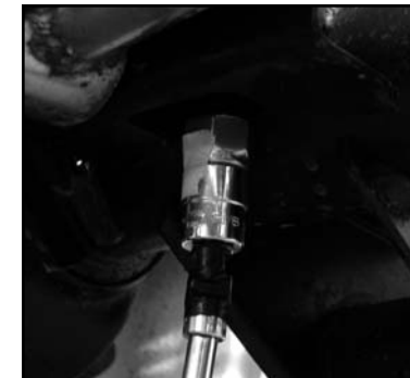
FIGURE 12.5 ADDITIONAL METHOD OF STARTING NUT ON FRONT LOWER RIGHT MOUNT
