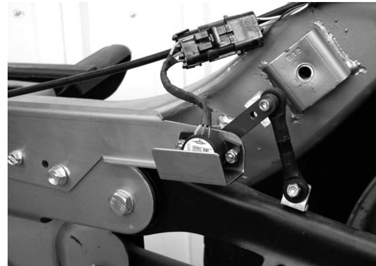
FIGURE 9.1 REAR RIGHT SENSOR SHOWN IN EXTENDED POSITION WITH ANGLE BRACKETS
