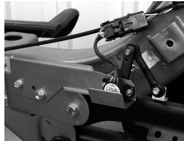
FIGURE 9.2 REAR RIGHT SENSOR SHOWN IN COMPRESSED POSITION WITH ANGLE BRACKET.
