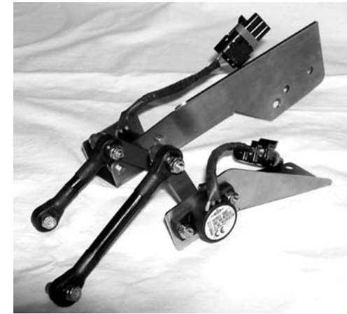
FIGURE 8.1 AiROCK™ HEIGHT SENSORS, FOR STANDARD LENGTH UPPER ARMS MOUNTED TO THE CHASSIS IN THE STOCK LOCATION.
