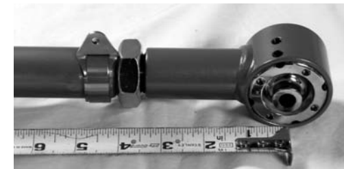
FIGURE 8.3 ROUND CONTROL ARM SHOWN WITH SENSOR LINKAGE MOUNT INSTALLED. NOTE 4 1/2" REFERENCE FROM CENTER OF PIVOT POINT
