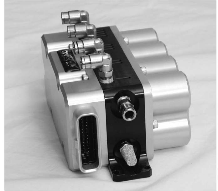
FIGURE 6.1 ACU SHOWING THE WIRE HARNESS CONNECTION, SINGLE AIR SUPPLY PORT, 4 AIRSPRING PORTS AND THE EX-HASUT MUFFLER
