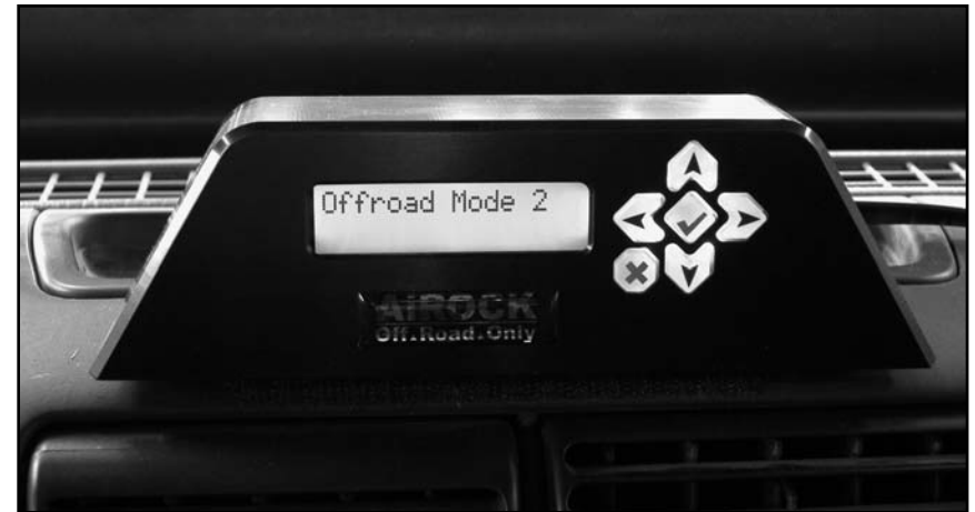
FIGURE 5.1 CONTROLLER MOUNTED IN RECOMMENDED POSITION ON CENTER OF DASH BEZEL
