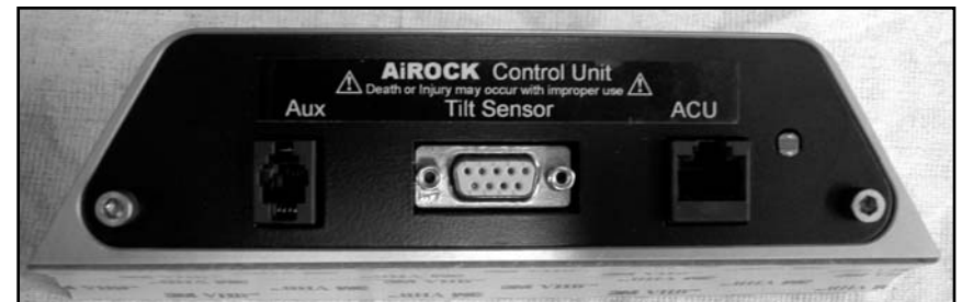
FIGURE 5.2 CONTROLLER BACKSIDE WITH CONNECTORS. PLUG THE FLAT BLACK RIBBON WIRE INTO THE PORT LABELED ACU. IN THE EVENT THAT THIS CABLE GETS UNPLUGGED, THE ACU NEEDS TO BE RESET BY REMOVING AND REPLACING THE INLINE FUSE. THIS WILL TURN THE CONTROLLER BACK ON.
